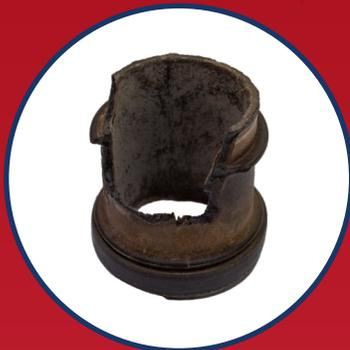
**Eliminate These Failures:** OEM doesn't hold on resulting in cracking and deformation.
